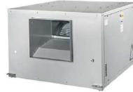
CEB - Certified Exhaust Box - 400°C/2h Tamaño/Size 9/4 - 30/14 Max 50.800 m 3 /h - 15 kW
